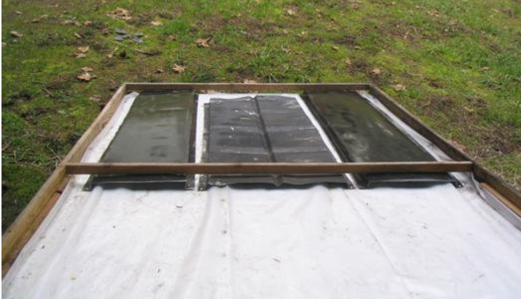
Figure 7. Another view of the air ducts shown without drying trays
