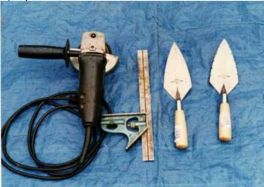
Figure 1. Angle grinder for modifying the trowel; masonry "pointing" trowel; and a weeding spade.
