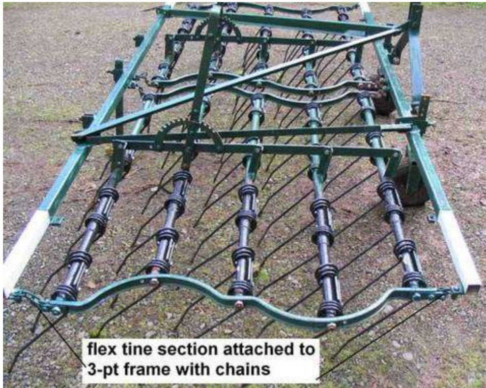
Figure 7. Flex-tine cultivator, side view.
