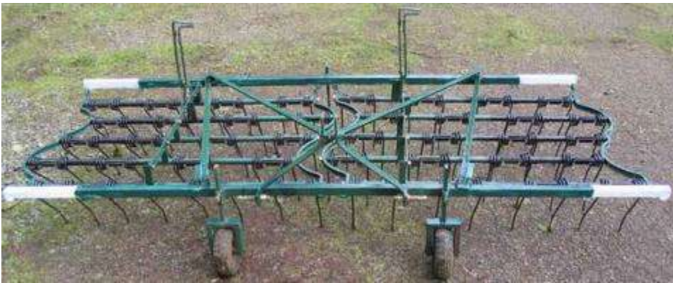
Figure 1. A 10 foot wide, 2-section flex-tine cultivator made from a spike-tooth harrow.
