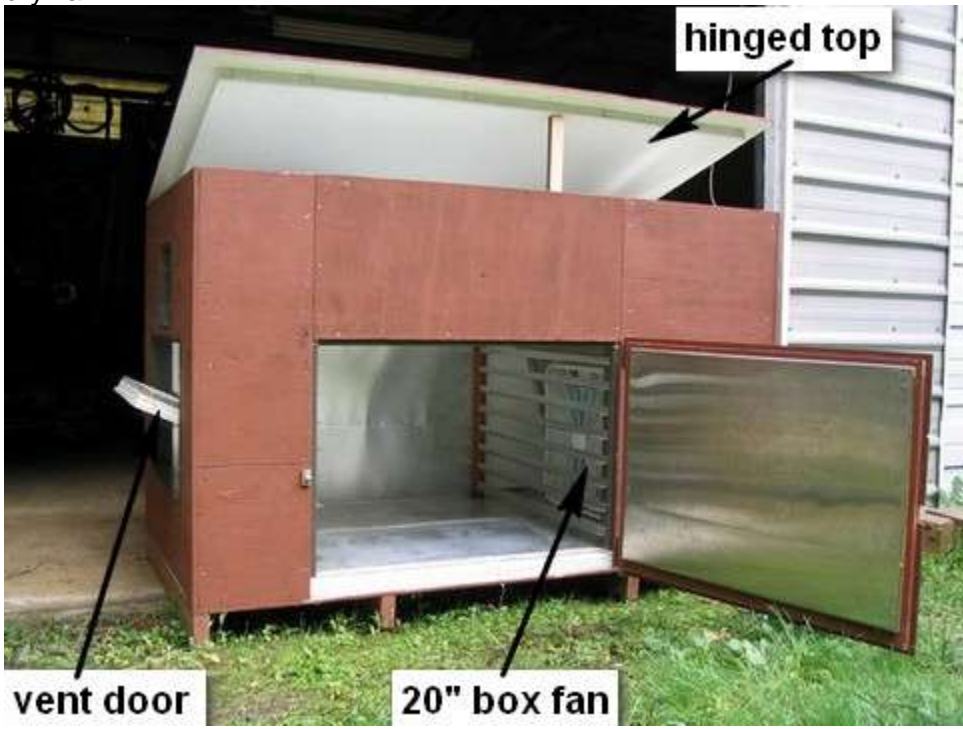
Figure 1. Food Dehydrator using 1/2 inch plywood, 2x2 and 2x4 frame and 1/2 inch drywall.
