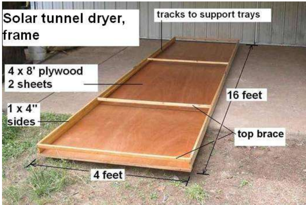
Figure 3. Solar tunnel dryer frame, 4 ft x 16 ft (1.2 x 4.9 m).
