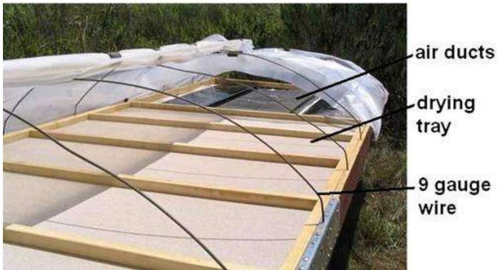
Figure 6. Air ducts convey heat under drying trays.
