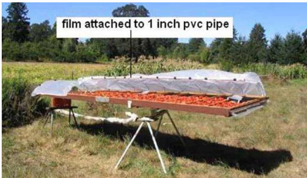
Figure 2. Solar tunnel dryer with tomatoes in drying trays.
